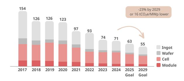
In 2024, our GHG emissions intensity was 71 tCO<sub>2</sub>e/MWp. While this fell short of our target of 69 tCO<sub>2</sub>e/MWp due to a lower-than-expected capacity utilization rate across our manufacturing sites, it still represents a 3 tCO<sub>2</sub>e (approximately 4%) reduction from our 2023 levels. This progress is largely attributable to the implementation of energy-saving and emission-reduction measures across our ingot, wafer, cell and module
